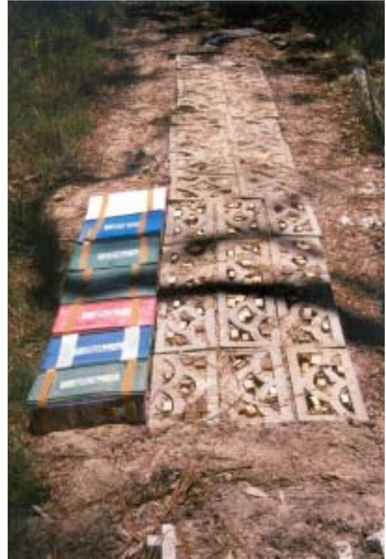
**Figure 3.** Concrete bricks were laid above the trench. Radiata pine feeder stakes were driven into gaps in the bricks to encourage movement of termites from the ground to the test specimens.
