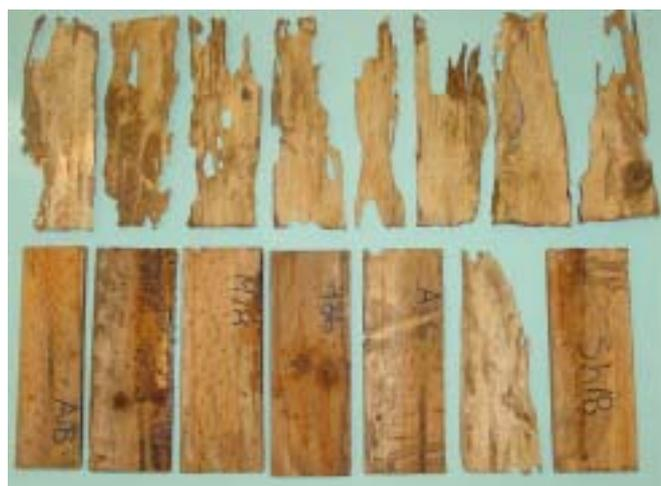
**Figure 7.** Damage caused by *M. darwiniensis* to feeder specimens (top row) and test specimens (bottom row): F<sub>1</sub> hybrid heartwood (4 samples), F<sub>1</sub> hybrid sapwood, slash pine sapwood and slash pine heartwood (left to right, respectively)
