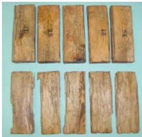
**Figure 5.** Damage caused by *M. darwiniensis* to maritime pine test specimens: heartwood (top row), sapwood (bottom row)
