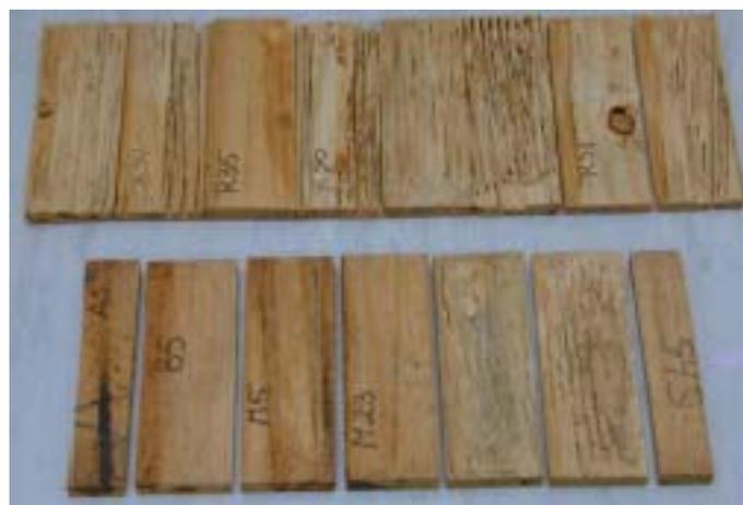
**Figure 6.** Damage caused by *C. acinaciformis* to feeder specimens (top row) and test specimens (bottom row): F<sub>1</sub> hybrid heartwood (4 samples), F<sub>1</sub> hybrid sapwood, slash pine sapwood and the slash pine heartwood, left to right, respectively)
