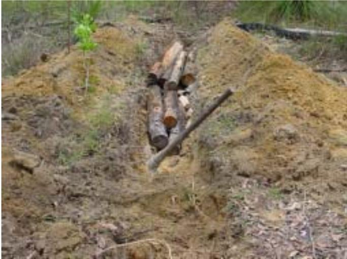
**Figure 2.** Trenches were filled with slash pine off-cuts and backfilled with soil to encourage sustained foraging by termites at Beerburrum and Townsville
