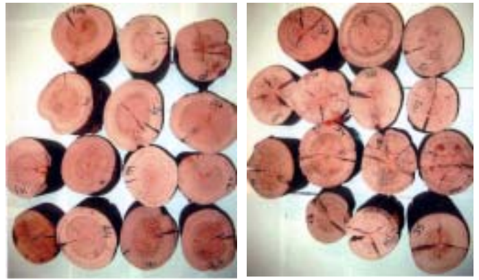
Figure 4. Differences in checking in the discs from low strain and high strain trees: <600 microstrain (left); >1200 microstrain (right)
