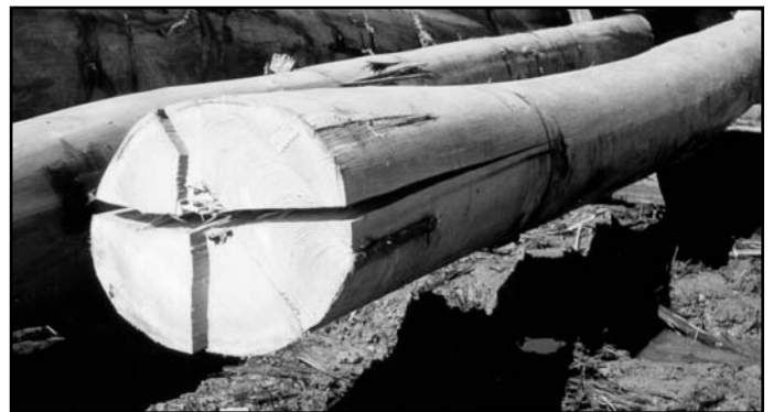
Figure 1. Log end splits due to the release of growth stresses following the crosscut ( Eucalyptus spp.)
